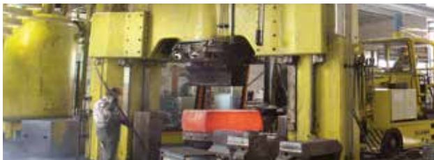
Open-die forging, hydraulic forging press
